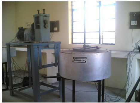
Fig 3: Shows Electrical Resistance Furnace
